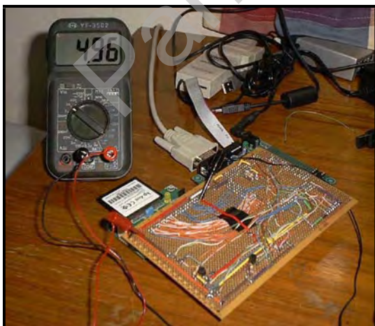
Figure 5-2 Multimeter used to test voltage level of I/O pin
